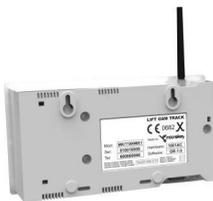
Before fixing the device in place, check the network coverage within the immediate environment. The Universal Gateway can be used as a coverage meter by connecting the battery cable to J3 and changing the jumper switch J10 to ON (see fig 1). The five LEDs on the front of the unit will show the network signal level. Once a suitable location has been found, switch J10 back to OFF.
